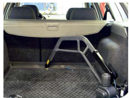
The hoist folded to the floor
